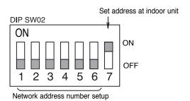
(3) Changing the SW02 position1 to 4 can set the address. The example below shows the address set at 16. The table on page?? shows the switch combinations for each address number.
