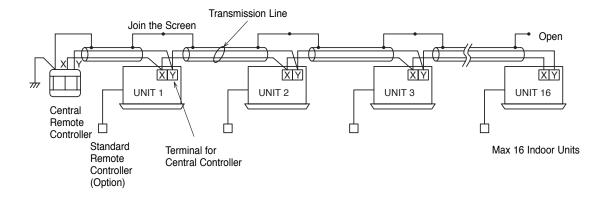
The screen for the transmission line is to be grounded only at the Central Remote Controller. The screen is to be joined at each unit but not grounded. At the last indoor unit do not connect the screen.
