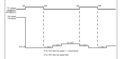
On receiving first release signal ON, the fan speed is changed from full speed to off.
