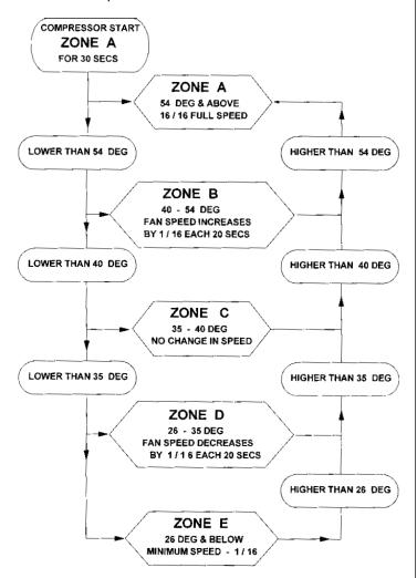
When the compressor starts, the fans assume the maximum speed for 30 seconds; at the end of this period, the fans come under temperature control. Below 26° the fans are at the minimum allowable speed, above 40° they run at full speed. The TL sensor temperature range from 26° to 54° is divided into three additional temperature zones:
