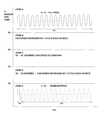
The sequence of switching is time and temperature based and is determined by the temperature detected at the TL sensor. The sequence is shown in below
